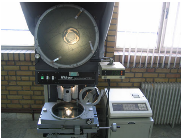
Fig. 7 The measurement technique by profile projector
